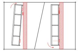
Hang the furniture unit on the top bar, allowing it to slide down into position. We recommend further securing the unit to the wall by driving 2 screws through the lower bracing bar.
